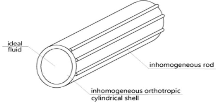
**Fig 2.1.** Inhomogeneous, fluid-contacting orthotropic cylindrical shell stiffened with inhomogeneous rods
