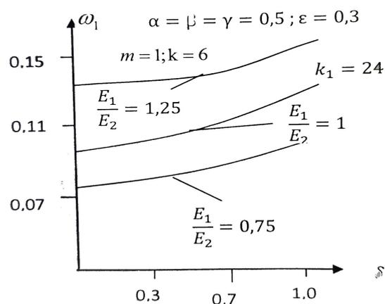
Fig. 4.1. Dependence of the frequency parameters on the number of rods
