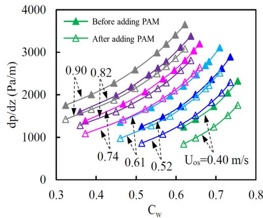
**Fig. 4. Effect of adding polyacrylamide (PAM) to the aqueous phase on specific pressure drop under the annular mode of oil flow in water**
