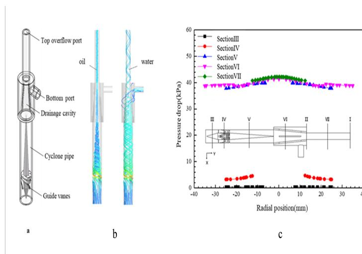
**Fig. 3. Lubricating elements - (a) structure; (b) streamline distribution; (c) resistance characteristics**
