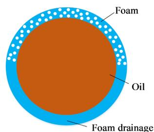
**Fig. 5. Degradation of oil ring flow in a water-foam ring**
