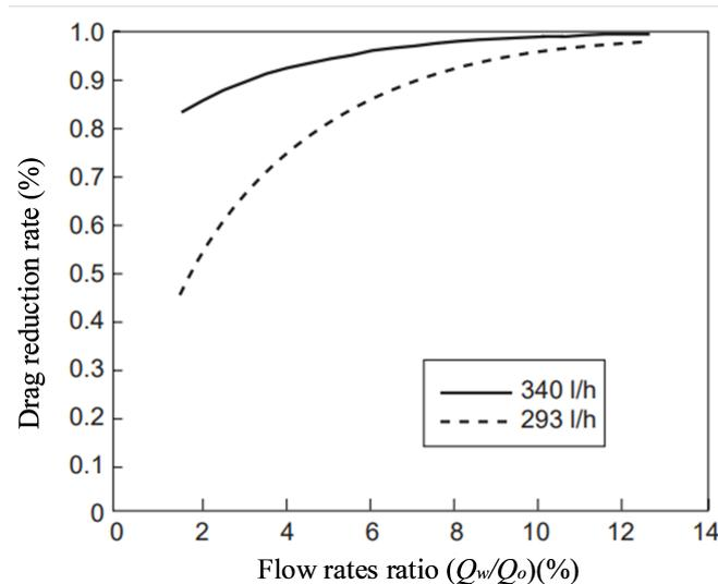
**Fig. 2. Effect of oil-water flow ratio on DR rate under fixed total flow rate**
