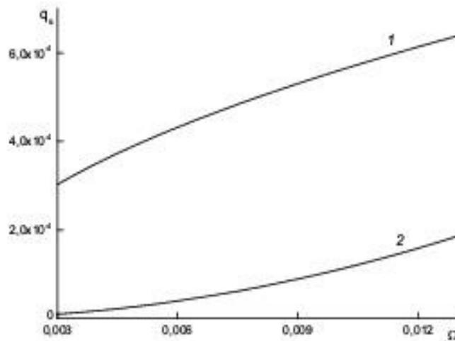
**Fig. 2** Surface absorption at  $\varepsilon = 0.0001$  and  $\alpha = 0$  in the case of mirror boundary conditions (1) and in the case of diffuse boundary conditions (2)
