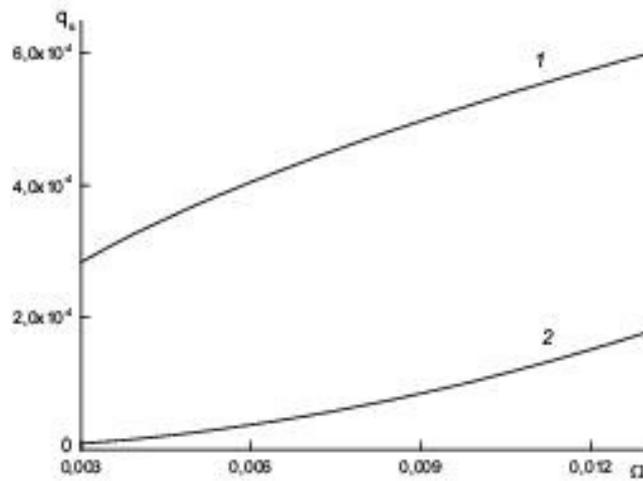
**Fig. 1** Surface absorption at  $\varepsilon = 0.0001$  and  $\alpha = -1$  in the case of mirror boundary conditions (1) and in the case of diffuse boundary conditions (2)
