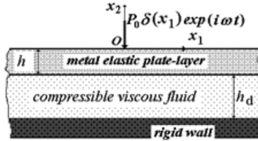
Fig. 1. The sketch of the hydro-elastic system under consideration
