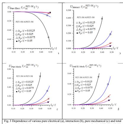
Fig. 3 Dependence of various pure electrical (a), interaction (b), pure mechanical (c) and total electro-mechanical (d) energies on the ratio  $\ell_0/\ell$  under various  $h_F/\ell$  for the PZT-5H/Al/PZT-5H plate.
