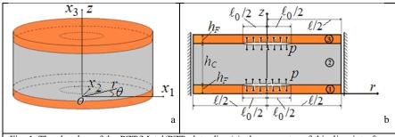
Fig. 1. The sketches of the PZT/Metal/PZT plate-disc (a), the geometry of this disc, interface cracks and external opening forces
