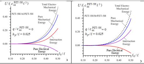
Fig. 2. Graphs of the dependencies between energies and the ratio  $\ell_0/\ell$  in Case 2 for the PZT-5H/Al/PZT-5H (a) and PZT-5H/St/PZT-5H (b) plates
