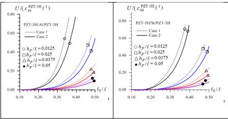
Fig. 4 The influence of the piezoelectricity of the face layers of the plates PZT-5H/Al/PZT-5H (a) and PZT-5H/St/PZT-5H (b) on the values of the total electro-mechanical energies obtained for various values of the ratios  $\ell_0/\ell$  and  $h_F/\ell$ .
